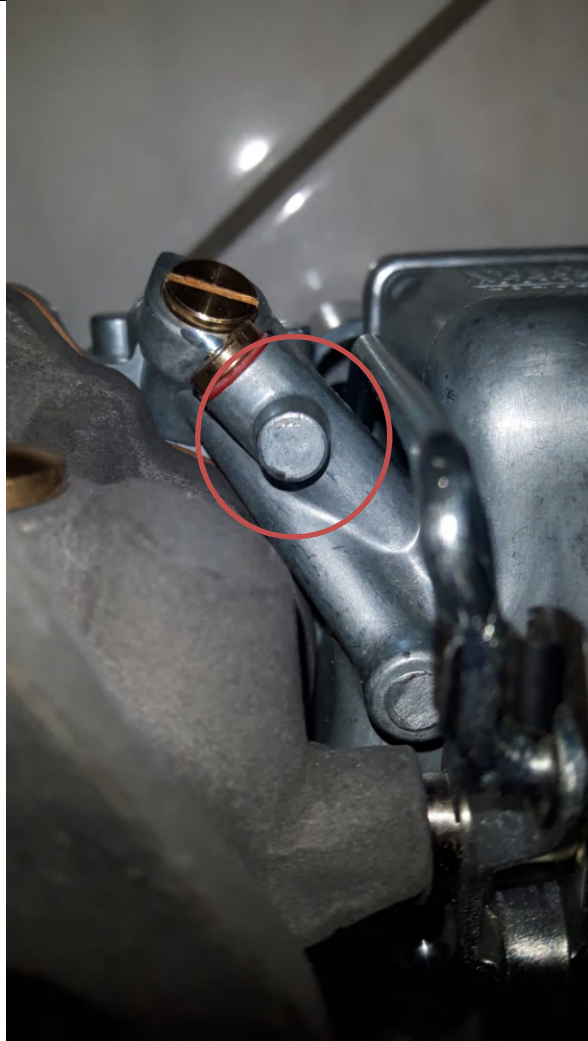
Casting in the area of the Idle-Speed is smaller in diameter, without an aluminium rivet.
