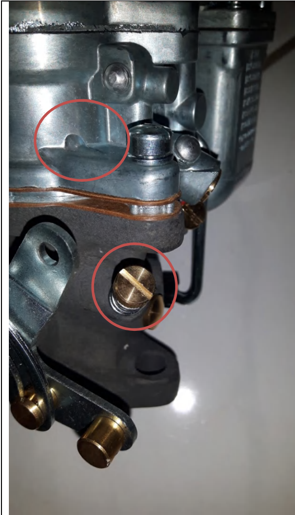
The markings on the idle-mix adjusting screw are missing, the reinforcing rib is not so prominent.
