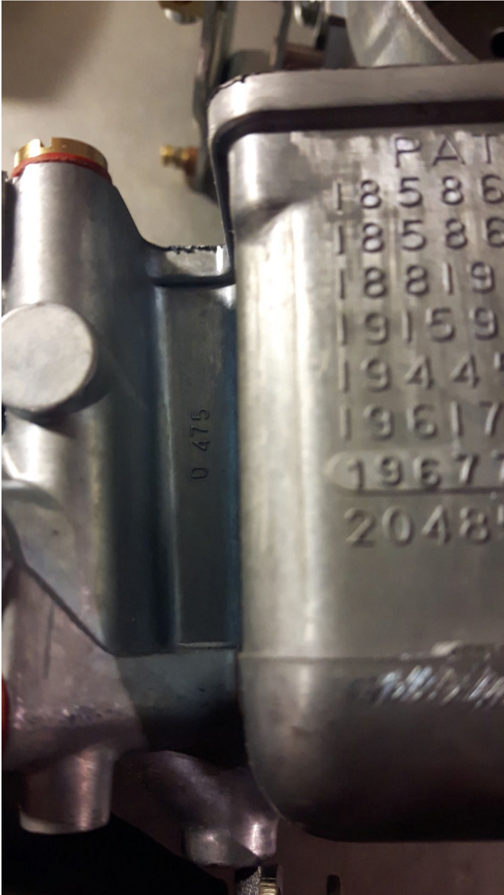
The bowl is correctly 0 475 marked with the correct 8 Patent Numbers.
