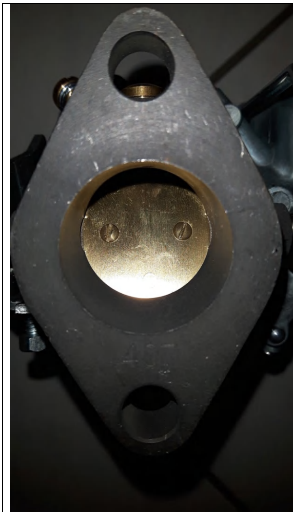
Butterfly valve is brass and only Circled C stamped.
