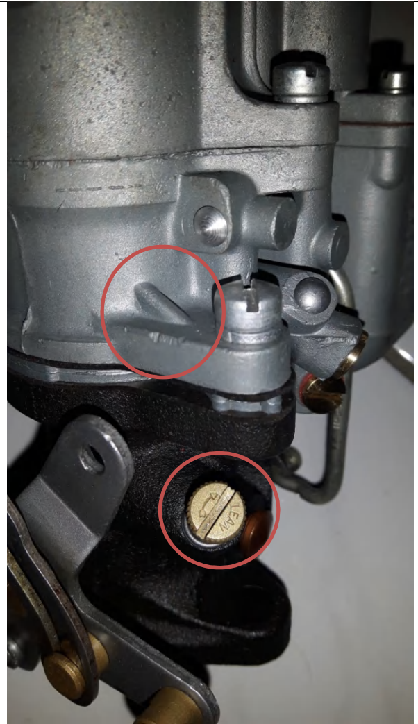
LEAN and arrow marking on the idle-mix adjusting screw, reinforcing rib is more prominent.
