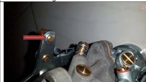
Washer is plated steel.
