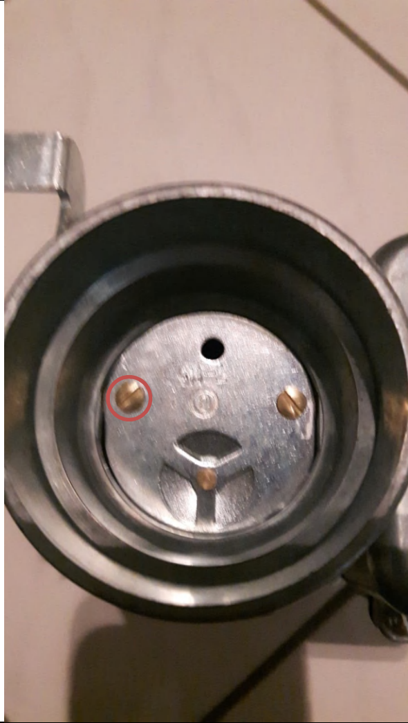
Choke Valve attached with a big flat slotted Post War screws.
