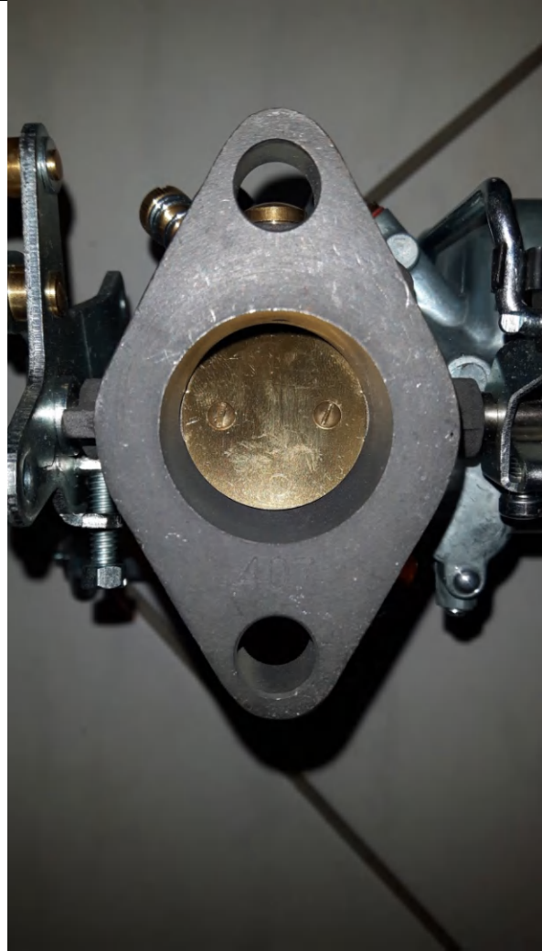
Base is only 407 stamped, additional markings are missing.
