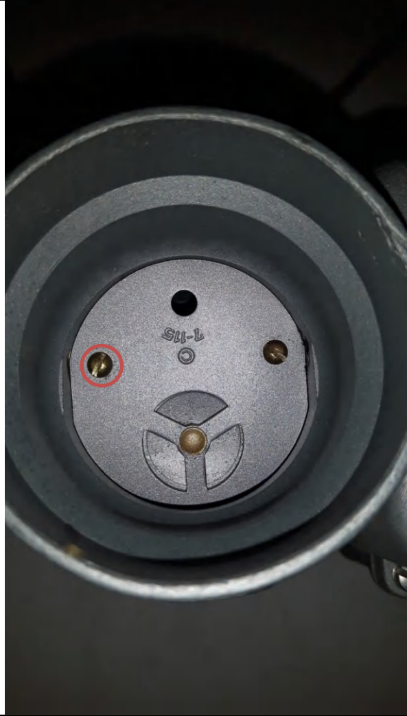
Original, small round head slotted screw. Different sizes of markings are on original plates visible too.
