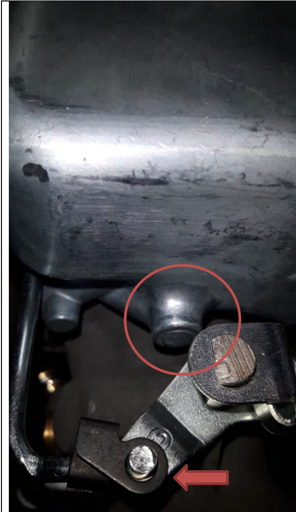
Different bowl casting in the High-Speed area.
